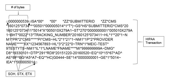
Figure 3. Example of TCP/IP Communication Transport Protocol Wrapper
